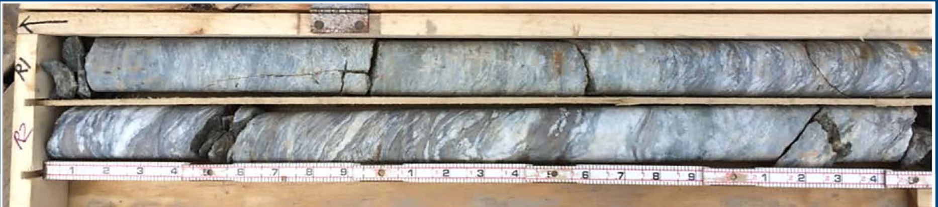
Photo 5: Core box containing dried core from test boring BB-BHF-202: Left side of core box (top 2.5-foot portion of cores).
