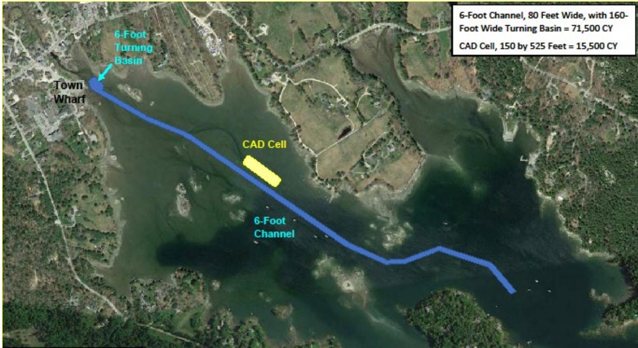
**Figure E-4: New Channel Showing Limits of Dredging**
