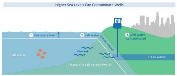
Fig. 4 Sea level rise and saltwater intrusion of well water (Carver and Shaffner, 2017)
