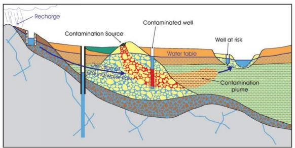
Fig. 2 Example of a contamination plume (MGS, 2005)
