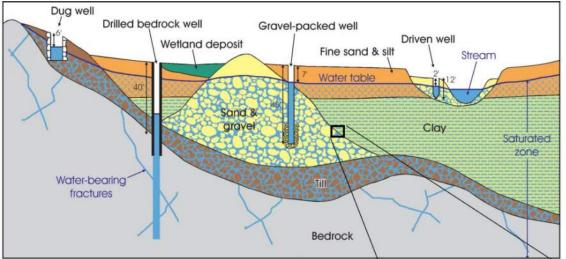
Fig. 1 Diagram of well types and aquifers (MGS, 2012)
